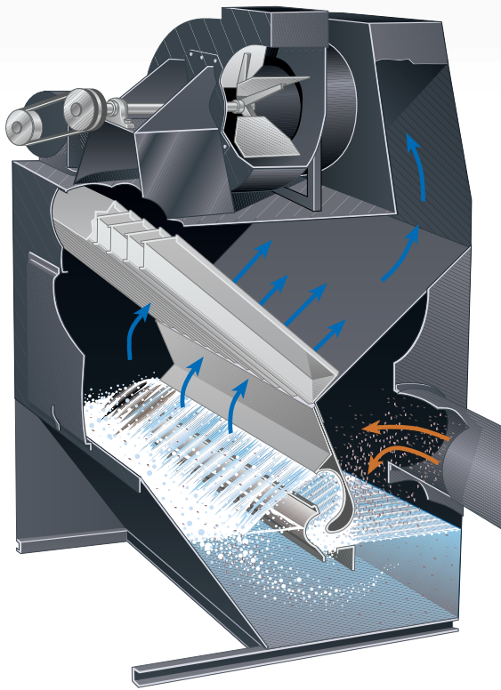
Arrangement B, Size 6 or smaller, wide-spaced chevron water eliminators remove entrained water from the clean air
