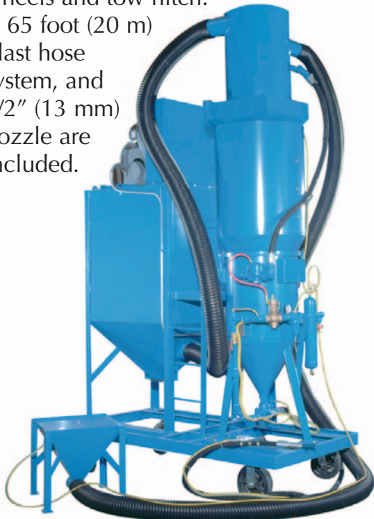
Cabinet Option with Accu-Flow Valve provides precise control for surface preparation of small parts.
